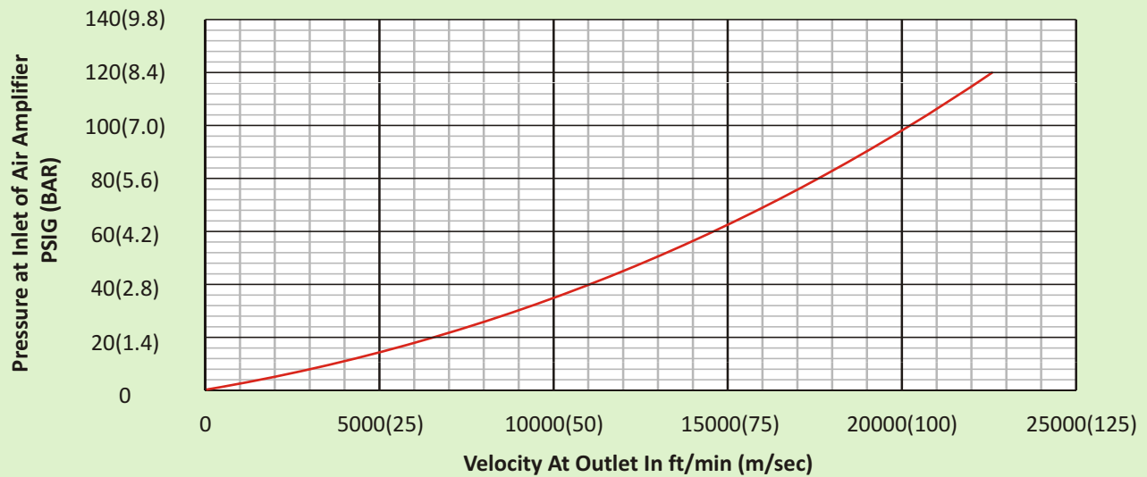
Pressure vs. Velocity At Outlet for Model 40002 & 40002S Adjustable Air Amplifier
