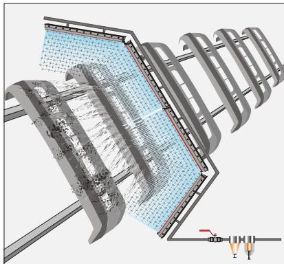
Three 24" X-Stream™ Air Blade™ Ionizers Blow off dust from Automotive Bumpers prior to painting. The NEX FLOW™ PLCFC controls the air on and off as required minimizing air consumption. In this case the static bars were "daisy-chained" together minimizing extraneous cable and reducing the number of power supplies needed.
