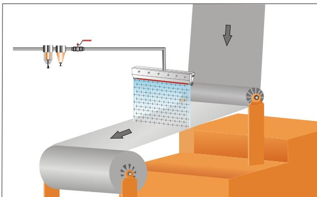
A Model 16118X removes static from extruded rubber web on a rewind. Previously the static charge was so high that any spark would cause the rubber to burn which regularly happens the 'extra strong' VS Bar combined with the X-stream™ Air Blade™ eliminated this unsafe situation.
