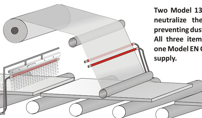
Two Model 13030 RN static bars neutralize the plastic laminate preventing dust attraction. All three item are connected to one Model EN C-4-4-outlet power supply.
